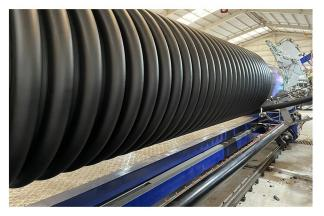
**Light and easy to handle** – A DN1500 ECOPIPE<sup>™</sup> pipe weigh-less in contrast to a 1500 Class 4 concrete pipe.
